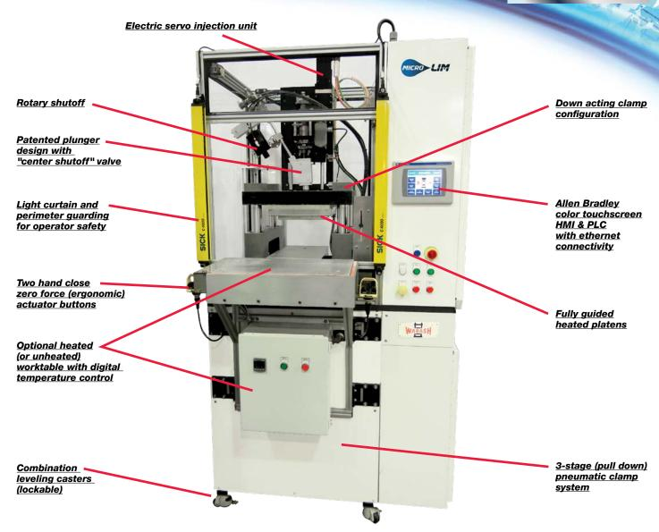
Ideal for clean room and medical applications, the hybrid servo-pneumatic MICROLIM™ Liquid Injection Molding Machine is designed for shot sizes from less than 1cc to 15cc. The MICROLIM features clamp force up to 17 tons and accurate shot size control from a patented plunger design with "center shutoff" nozzle.
